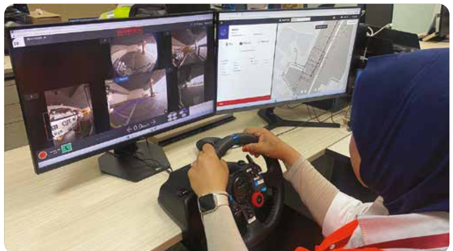
The autonomous vehicle fleet supervisor could take control of the vehicles remotely, where needed, to manoeuvre around obstacles.
