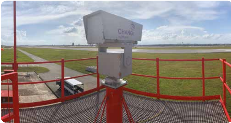
iFerret provides automated round-the-clock surveillance of the runway to reduce the threat of foreign object debris.
