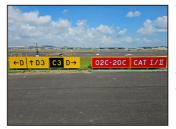
White-on-red mandatory signs are also located at ILS CSA holding positions. These signs warn drivers and aircraft that the ILS CSA is ahead. When the ILS CSA is active (i.e. the red stopbars are switched on), drivers shall obtain permission
