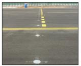
The holding position is a dashed white or yellow line marked across the taxiway, located near taxiway intersections. It is a designated position intended for traffic control at which taxiing aircraft and vehicles shall stop and hold until further cleared to
