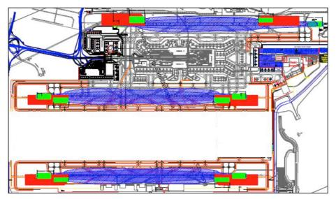
CSA (indicated in red and green above) are areas where the presence of vehicles may interfere with signals required by pilots for precision approach landings. Vehicles must stay clear of CSA. To enter CSA, permission must be sought from ATC.
