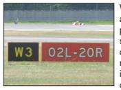
White-on-red **mandatory signs** are located at runway holding positions (explained in a later section). These signs warn drivers and aircraft that the runway indicated on the sign is ahead; drivers shall exercise caution so as not to inadvertently
