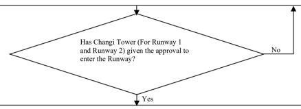
ATC upon giving clearance, shall simultaneously turn off the red stopbar lights.
