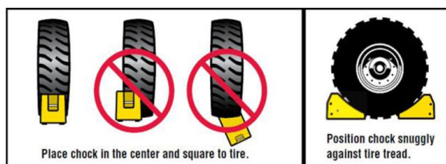
Sample of proper wheel chock placement
