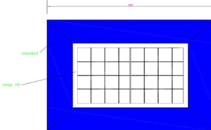
Picture 2 - Typical Installation with a slope of 45° (Top View)
