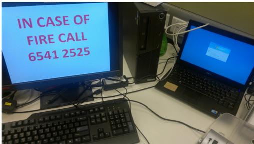
Where possible, all electrical equipment and their power outlets should be switched off when not in use to reduce component wear and tear, possible overheating and fire. Computers on 24 hr operations should be switched off for at least 1 hr per day to prevent overheating.
