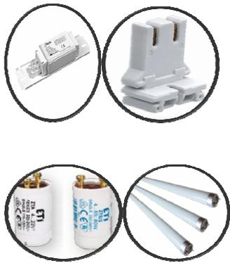
Lighting ballasts should be replaced according to the manufacturer's or qualified electrician's recommendation. Light bulbs/tubes should fit tightly into their sockets to prevent arcing. Wattage rating of the light starter and light tube should match. Light bulb/tube found discoloured i.e. bright yellow/orange/brown/ black should be replaced immediately.
