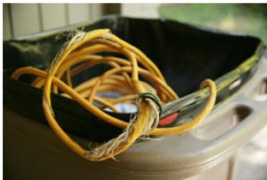
Check and replace cracked, damaged or loose electrical plugs, cords and connections. If you have older cords with cloth covering, check for and replace frayed cords.
