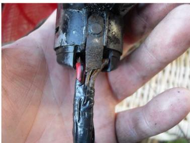
Never use tape to connect or secure electrical fittings, wirings or connections.
