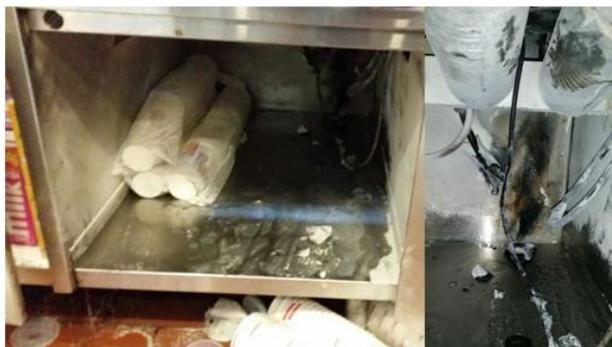
Fire at T2 on 11 Oct 2014. Investigation found fray wiring which might be the cause of the fire.
