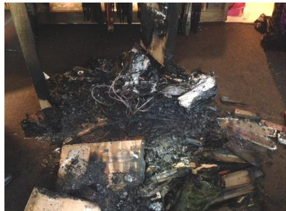
Fire at T3 on 13 Oct 2014. Investigation determined that the origin of the fire was from the electrical wiring below a carpet where the display cabinet was placed.
