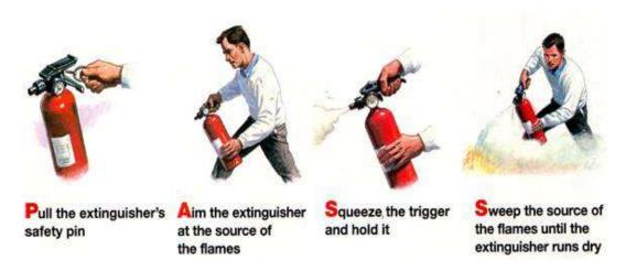
For trolley extinguishers, the method of application is similar to that of the portable extinguisher; the only difference would be a need to open a valve after pulling out the safety pin (Step 2 in the diagram below). Refer to the diagram below for the step by step description of how to operate the extinguisher.
