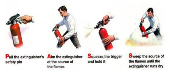
4.5.4 For trolley extinguishers, the method of application is similar to that of the portable extinguisher; the only difference would be a need to open a valve after pulling out the safety pin (Step 2 in the diagram below). Refer to the diagram below for the step by step description of how to operate the extinguisher.
