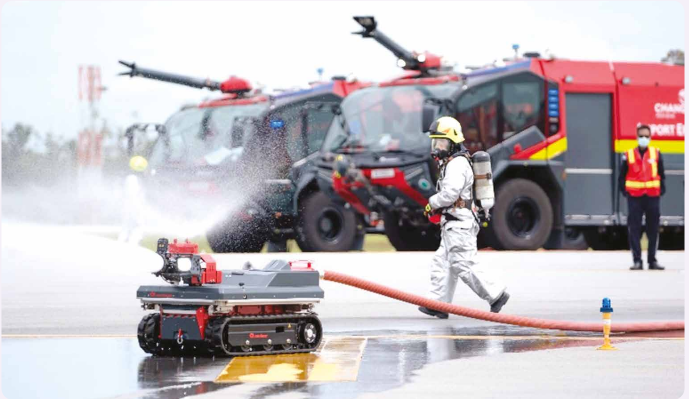
>> New solutions, such as firefighting robots, were trialled at Exercise Bobcat to improve firefighting capabilities.
