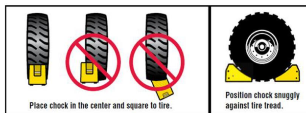
Sample of proper wheel chock placement
